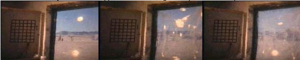
Laminated window exposed to blast pressures.
