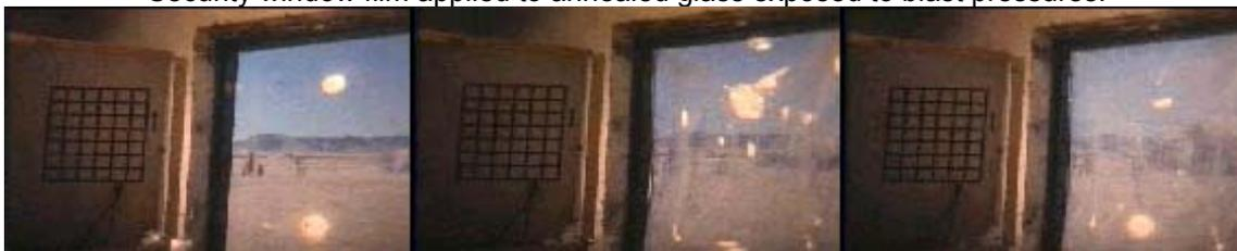
Laminated window exposed to blast pressures.
