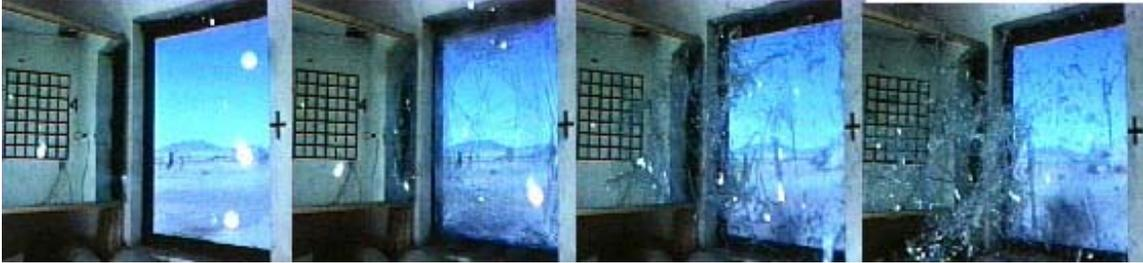
Unprotected annealed glass exposed to blast pressures.
