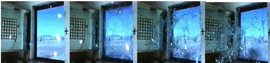
Unprotected annealed glass exposed to blast pressures.
