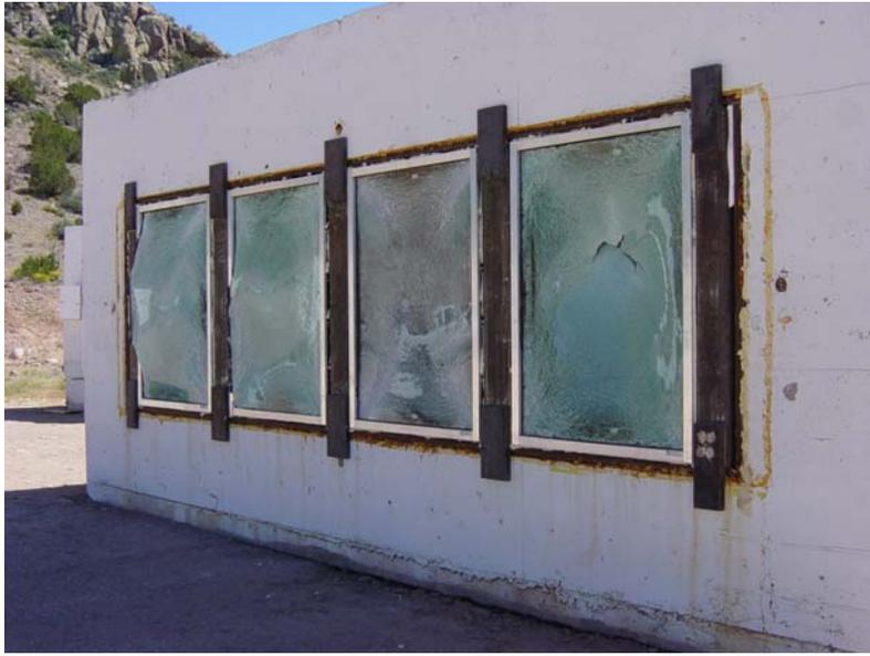
**Figure 8. Post-Test Photo of Thick Laminate Window System Response.**
