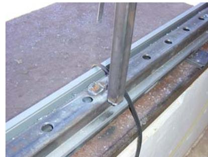
**Figure 6. Failure of Standard Muntin End Connection.**
