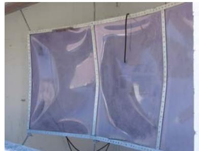
ABOVE: 3/8" PVC material attached to steel frame and supported by steel rods. The rods were then attached to steel plates at the floor and ceiling by clevises.
