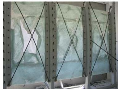
ABOVE: Pre-drilled SGP laminated glass panels attached to steel frame members and bolted to tube structure. Steel rods were introduced to determine their effect on the performance of the retrofit design. While effective they were found to be unnecessary.
